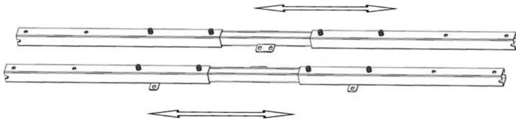
1. According to the demand of the panel adjust the frame length
