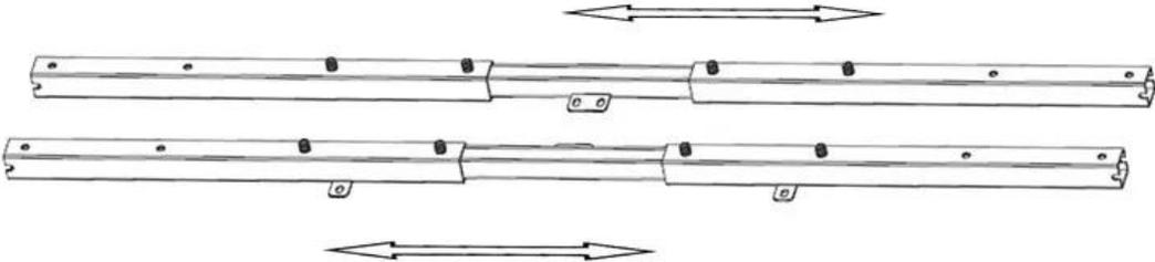
1. According to the demand of the panel adjust the frame length
